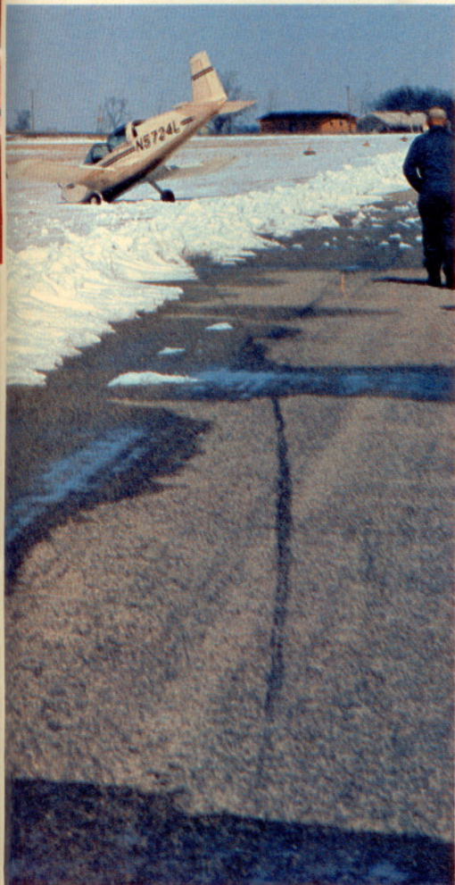
This tire mark on the runway surface led the pilot to believe, at first, that his left brake locked on touchdown. Investigation showed nothing wrong with the brakes and pilot learned more than one thing could have caused tire mark.
